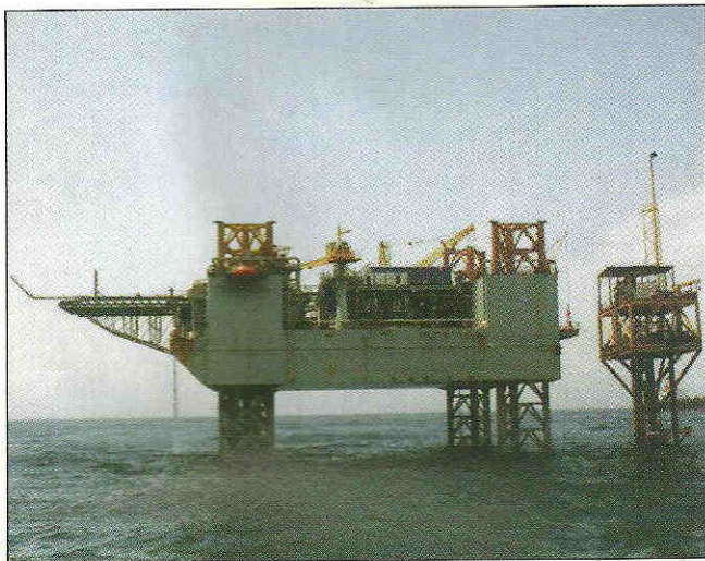
On our cover: Jack-up Gulftide was converted into MOPU in just 122 days to meet a gas delivery deadline. The trend to recycle elderly drilling units into production units is keeping rig market tight in U.S. Gulf and worldwide (p 17)
