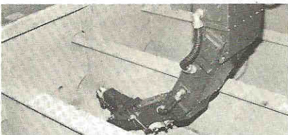
Painting robot, result of Japanese shipbuilding research (p.64)
