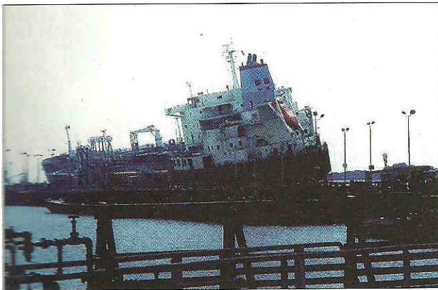
Some new-generation double hull tankers have suddenly tilted during operations at terminals. A SNAME panel has investigated why this happens and made recommendations to prevent such incidents in future (p. 40)
