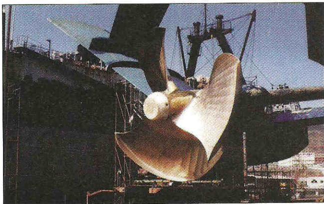
One of a pair of 1 m diameter CLT propeller units fitted to the 34 knot hydrofoil Barracuda . Owner Trasmediterranea now intends fitting CLTs to its other hydrofoils (p. 27)
