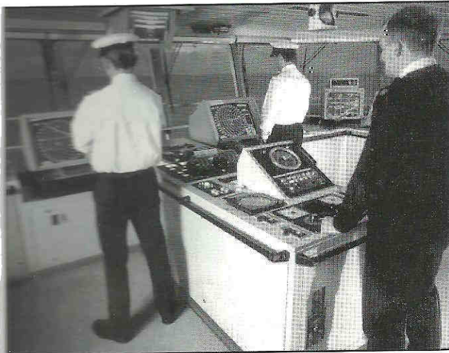
Electronics outfit of ship pictured on our cover includes a Racal Recorders VER (Voyage Event Recorder)—a “black box” that keeps a continuously updated record of radar, gyro heading and other data
