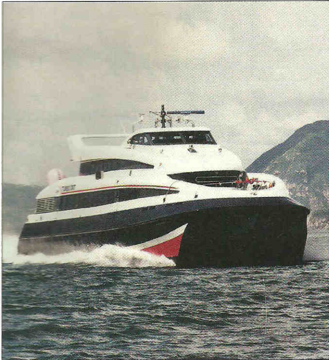
FBM Tricat design, powered by Solar gas turbines is being built under license by new Pequot River Shipworks in New London, Conn., one of several U.S. yards offering established international designs to meet a growing demand for fast, high passenger capacity ferries capable of open-water operations
